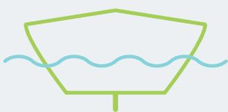
The flat bottom hull gives a greater surface area of contact between the ship and the water. This causes a greater displacement of water and leads to a stronger buoyancy force acting on the ship and therefore means it can take a bigger load. However, a flat bottom ship is less stable in large waves as it causes the boat to travel on top of the waves, instead of going through them.
