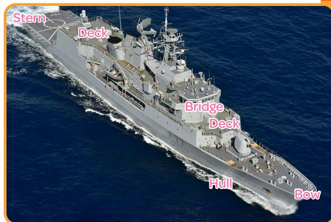
The weight of the ship is due to its **mass** and the **force** pushing down on it due to **gravity**. As the force due to gravity pushes the ship down it pushes aside the water to make room for the ship, this is called its **displacement** or **weight**. Navy ships are made from steel metal which is very heavy so they have a large weight/displacement.
