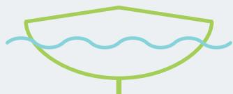
A round bottom hull is smooth and has less surface area in contact with the water than a flat bottom. Therefore, the buoyancy force is less so it can only take a small load, but it has low water resistance so it can go faster. Round bottom hulls are more unstable so they are prone to rocking and capsizing.
