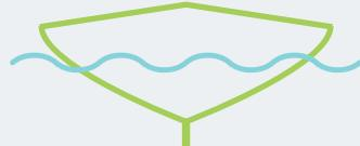
A v-shaped hull decreases the surface area of water in contact with the ship. This decreases the buoyancy force acting on the ship. It also reduces the friction, or water resistance, so the ship can go faster through the water. A v-shaped hull causes the bow of the ship to pierce through the waves rather than go over them so increases stability in rough water. Navy ships have a v-shaped hull.
