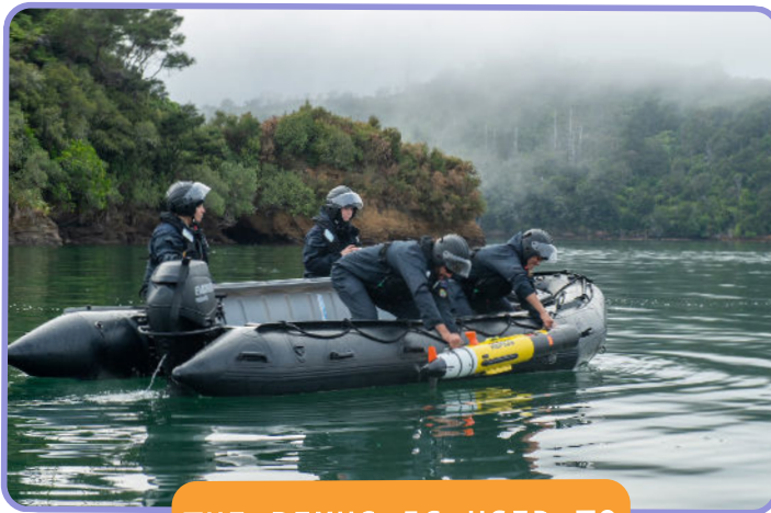
THE REMUS IS USED TO SURVEY THE SEAFLOOR
